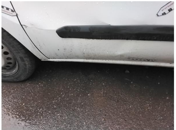
6: Door nsf Dented Over 30mm
