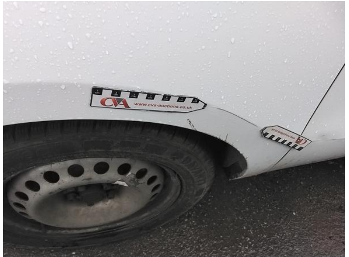
4: Wing nsf Scratched Over 25mm Thru Paint
